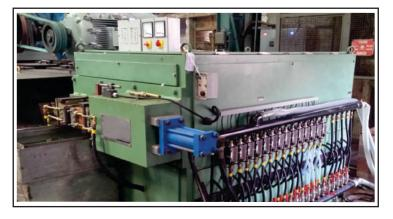
We possess expertise in manufacturing Copper Flexibles & Shunts of a wide range. We have Press-Weld Solidification Machine up to 250 KVA to produce a versatile range of Copper Flexibles, Shunts & Jumpers.
